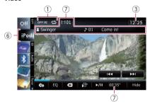
Playback condition indicator Indicates the current playback condition.
